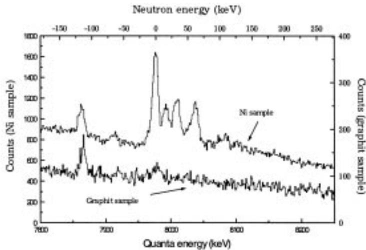
**Figure 7.** Experimental  $\gamma$ -ray spectra with Ni (effect) and graphite samples (background). Lower scale — for  $\gamma$ -quanta energy, upper scale — for energy of neutrons.
