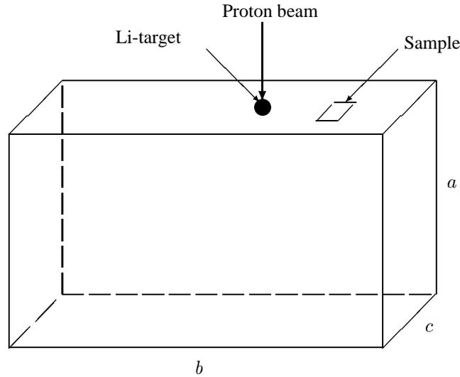
**Figure 5.** Positioning of the Li-target and the sample on a graphite prism for generating Maxwellian neutron spectra with  $kT = 10-15$  keV.
