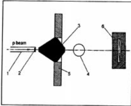
**Figure 6.** Geometry of the experimental setup for neutron spectrometry by means of the shift of primary  $\gamma$ -transitions. 1 – ion guide, 2 – Li-target, 3 – Pb shadow shielding, 4 – Ge-detector, 5 – sample, 6 – neutron monitor.
