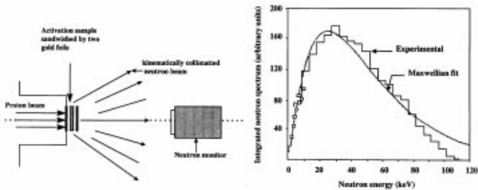
**Figure 4.** Experimental set-up (left) and Maxwellian neutron spectrum from  $\text{Li}(p, n)$  reaction on Van de Graaf at  $E_p = 1884 + 30$  KeV (right).
