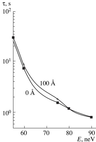
**Fig. 5.** Lifetimes of neutrons with energies above the boundary value, computed by the Monte Carlo method, as a function of their energy in the proposed geometry of the spectrometer for different values of oil-film thickness (figures near the curves) at the surface of Al membrane. The chamber dimensions are  $14 \times 14 \times 20$  cm. The UCN loss factor in collisions with the walls is  $\eta = 2 \times 10^{-4}$ ; the boundary energy is 200 neV.
