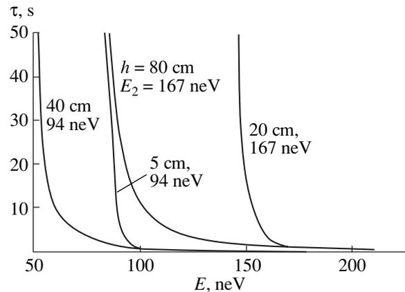
**Fig. 7.** UCN lifetimes in the neutron guide, simulated by the Monte Carlo method, versus their energy for different positions of the analyzing membrane.  $E_2$  is the boundary energy for membrane 8.
