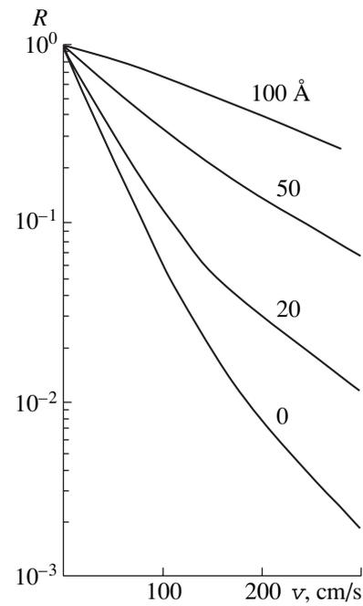
Fig. 2. Neutron-reflection coefficient  $R$  of polyethylene, obtained from the quantum-mechanical calculation, versus the normal component of neutron velocity  $v$  under different assumptions on the film thickness (figures near the curves) of Fomblin (fluorocarbon polymer oil, boundary energy 106 neV) on the polyethylene surface.
