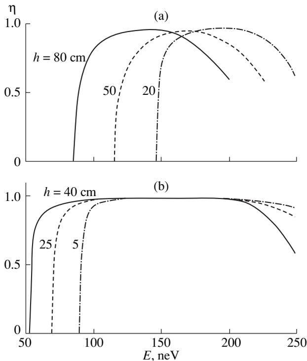
**Fig. 6.** Detection efficiency, simulated by the Monte Carlo method, for UCN scattered in the chamber as a function of their energy for different positions of the analyzing membrane (figures near the curves) (a) made of copper and (b) with Ge coating.
