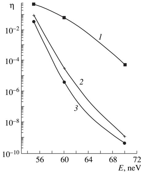
**Fig. 4.** The degree of “survival” of neutrons with energies above the boundary value within a time of 55 s with (1) polyethylene with a 100-Å oil film on the surface, (2) unpolluted polyethylene, and (3) ideal absorber used as spectrum formers.
